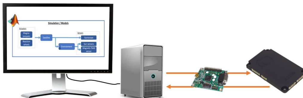
Figure 1: ADCS "Hardware in the loop" test bench
