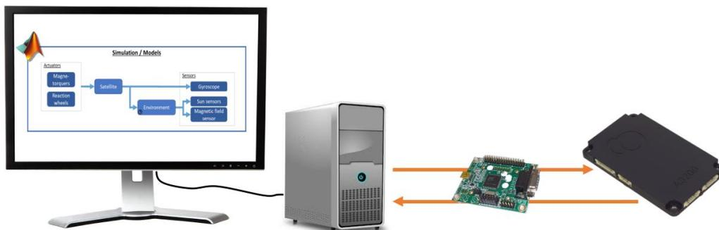
FIGURE 1. ADCS "HARDWARE IN THE LOOP" TEST BENCH
